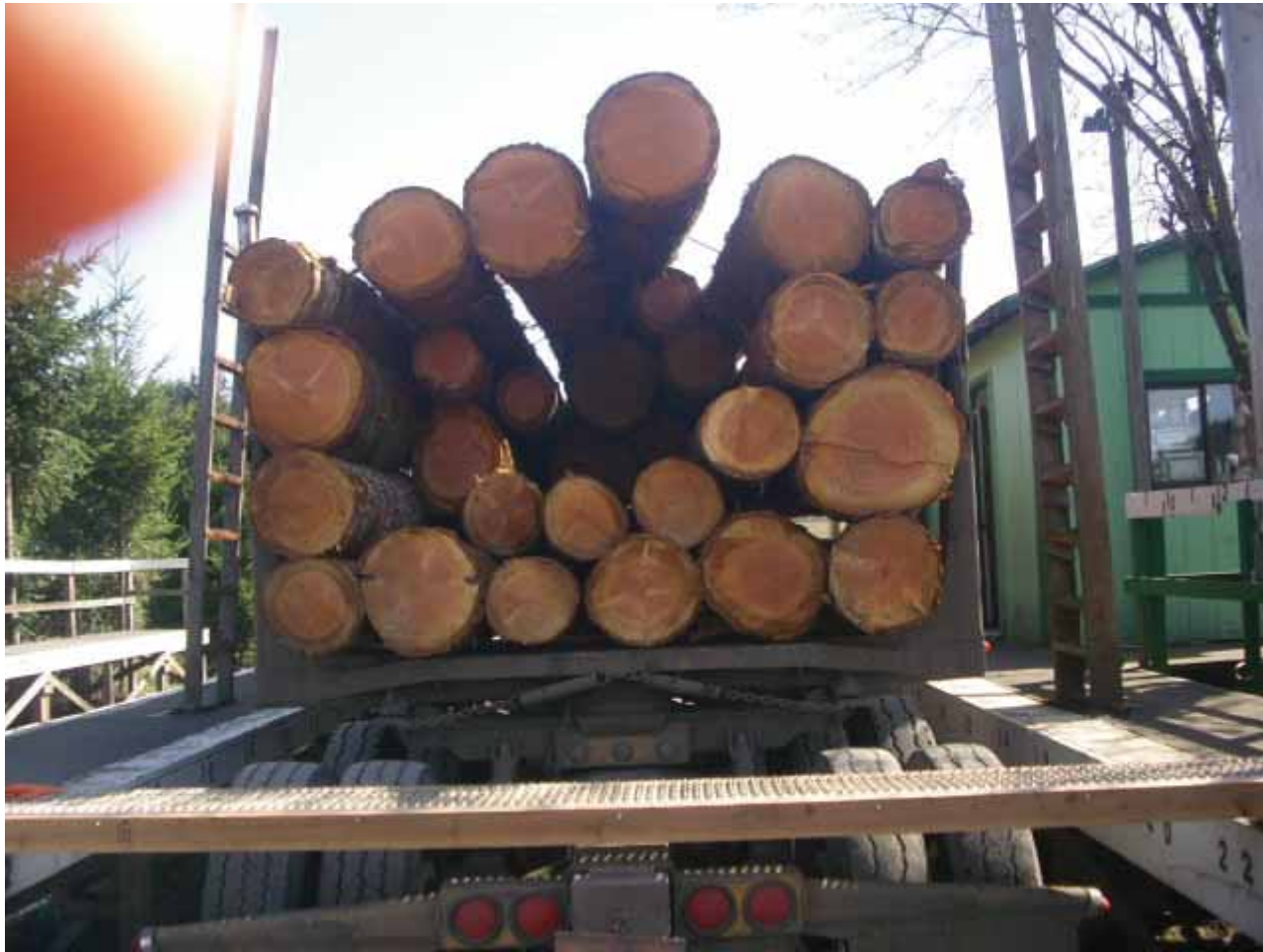
Short logs covered with long logs.
