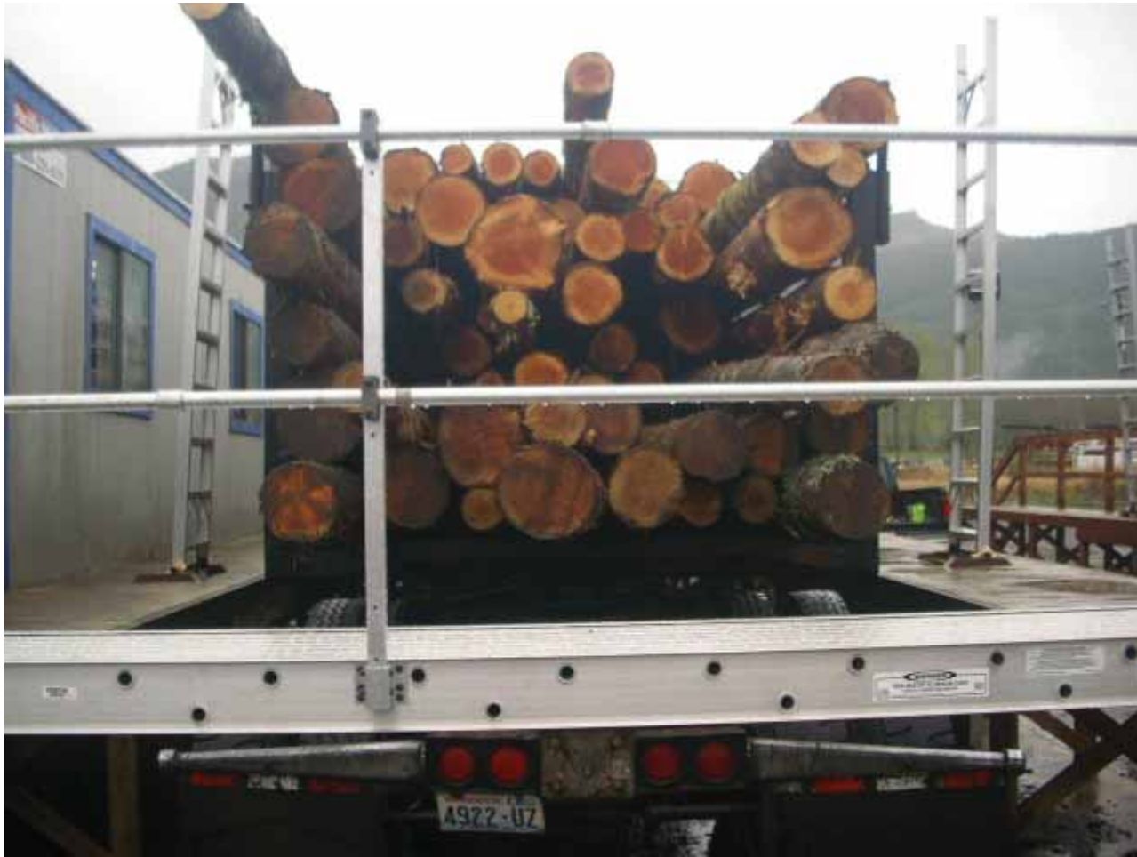
A drop plank at the rear of the truck provides a walk way across the rear of the load.
