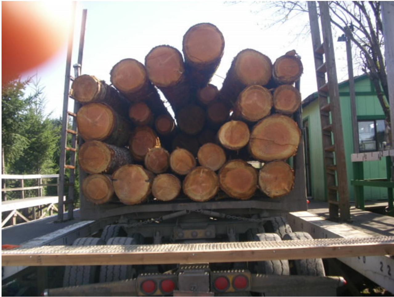
Short logs covered with long logs.
