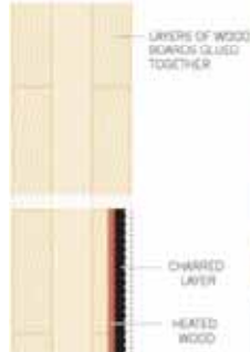
STRUCTURALLY SOUND CORE
