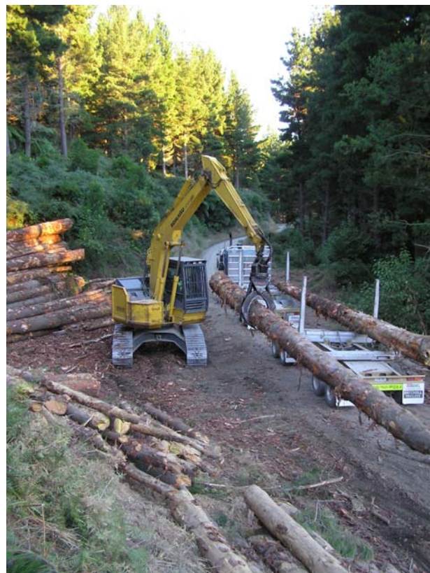
In forest 18m stem loading. Reduced landing requirement.
