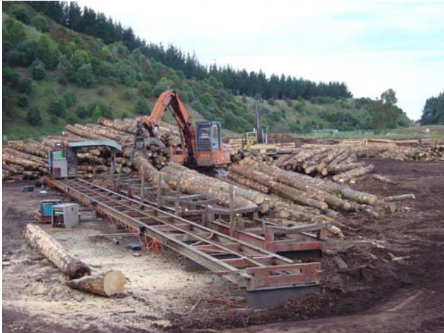
Scanner bed and log cradle in a yard setting. Secondary machine loading and unloading cradle. Logmaister processing head in background.
