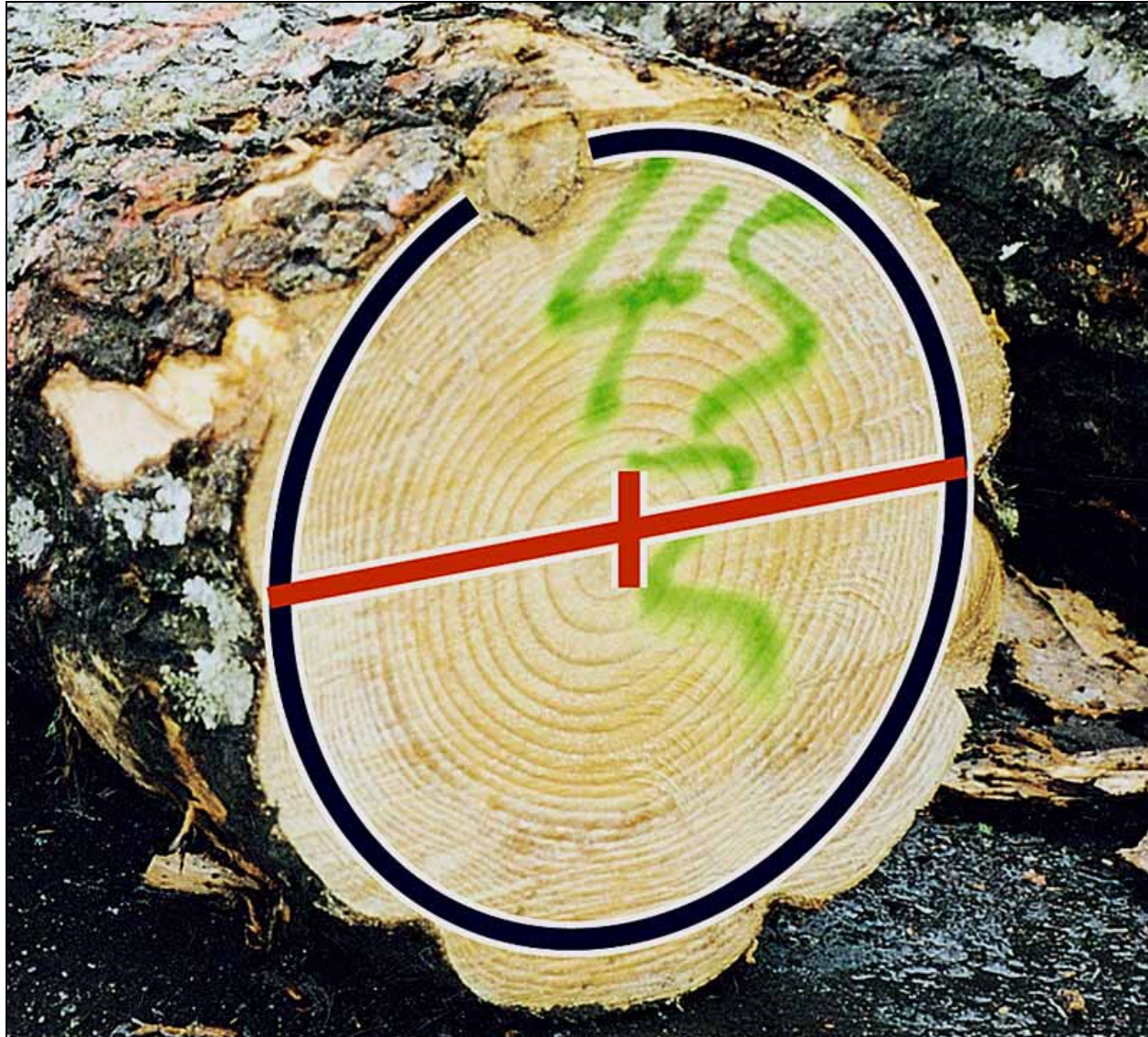
Fig. 11: Small-end swelling with bark-encased knot. This does not affect measurement, but swelling and fluting do.
