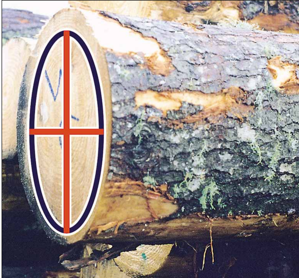
Fig. 7: Trumpet. Small-end diameter is reduced to exclude swelling.
