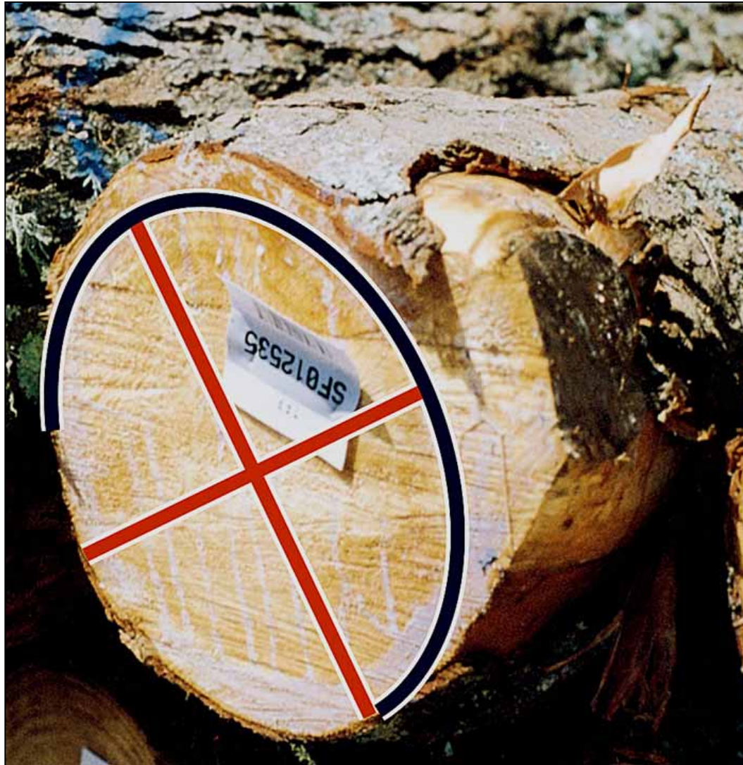
Fig. 13: Small-end swelling with intergrown knot. Swellings are excluded from measurements.
