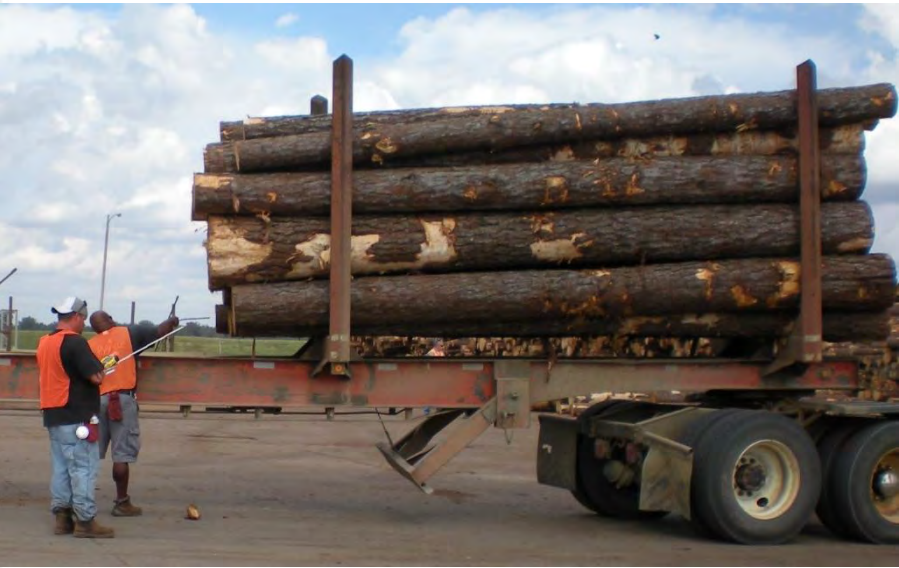
In the US South log inspection is on the truck at the scale
