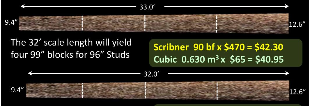
A mill cutting 92 5/8" PET studs would prefer a 31' scale length to yield four stud blocks without sending excessive wood to the chipper
