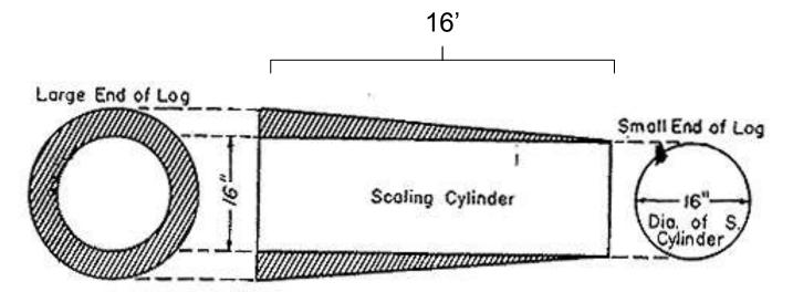
The 120" of surface area from the previous slide is converted to feet by dividing by 12" per foot, so 120" / 12" = 10 feet. The 10 feet are then multiplied by the segment length of 16 with a result of 160 board feet (bf). This gives an estimate of what can be sawn from this log segment, given the assumption applied to the diagram in terms of board feet which is a unit 1" X 1" X 12".
