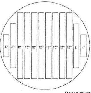
The end view drawing or diagram yields a surface area of 120" of 1" wide board at least 4" wide and accounting for 1/4" saw kerf between boards and wasting slab areas.
