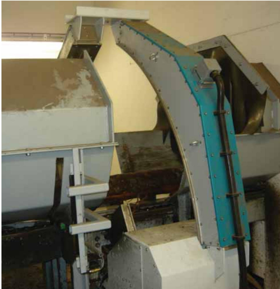
TOMOLOG: X-RAY SCANNING FOR DETERMINING INTERNAL WOOD CHARACTERISTICS
