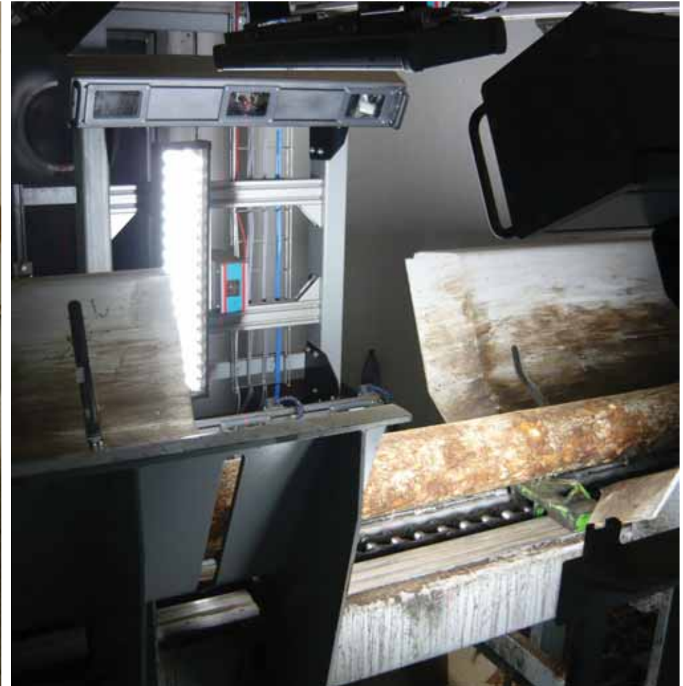
SCREENLOG-PLUS: COLOR SCANNING AND LASER TRIANGULATION FOR 3D RECONSTRUCTION
