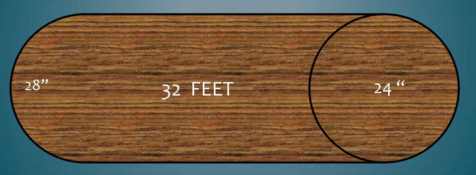
LENGTH DEFECT DEDUCTION OF 8 FEET DIAMETER DEFECT DEDUCTION OF 2 INCHES
