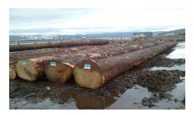
You can see in this picture that the scaler has put a Green dot (sort mark) of paint to separate out this log.
